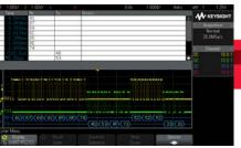
Serial bus triggering and hardware-based protocol decoding means you can efficiently debug your embedded designs that include serial bus communication.
