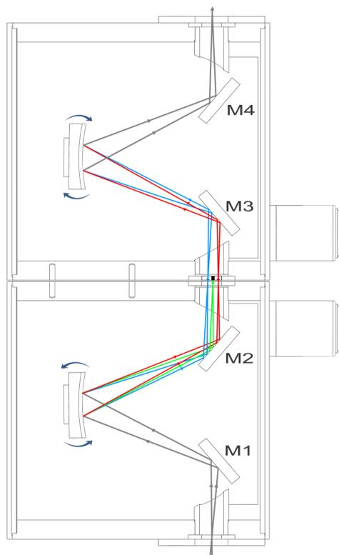
The 9030DS (Double Subtractive) is made of 2 back-to-back 9030 monochromators in a **subtractive** mode: the dispersion of the second monochromator is in the opposite direction of that of the first one. The gratings are calibrated to rotate synchronously in opposite directions.
