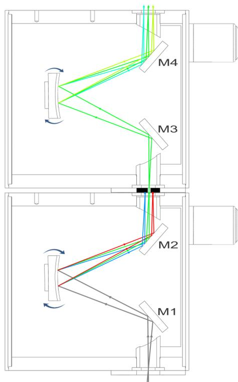
The 9030DA (Double Additive) is made of 2 back-to-back 9030 monochromators in an **additive** mode: the dispersion of the second monochromator adds to that of the first one. The gratings are calibrated to rotate synchronously in the same direction.
